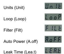
To select a menu item, press the SEL button. The display will then show the options. The menu button is used to scroll through the options. When the desired option is displayed press the SEL button to select and save it. The display then returns to the normal pressure or loop current mode.
