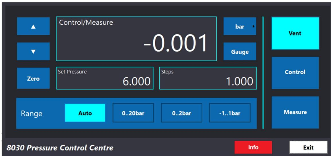
The display is designed for touch screen use, keyboard entry and using the CCPAD on CalBenches.
